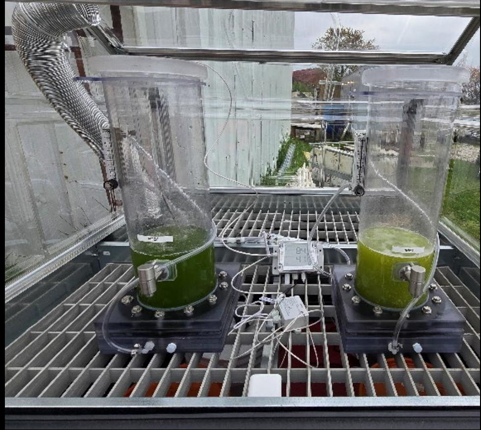
9-L Bioreactor tests
