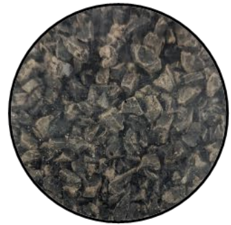
(a) Granulated Filler/HDPE Pellets
