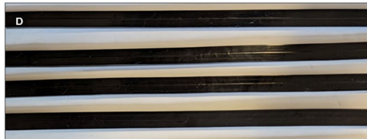
A. Reza holding an 80 wt.% filler ShAPE composite extrudate; B. Tooling cavity designed for manufacturing composite 'bars'; C. Cold-pressed composite feedstock granules in ShAPE ring; D. ShAPE polymer composite bars with no surface defects
