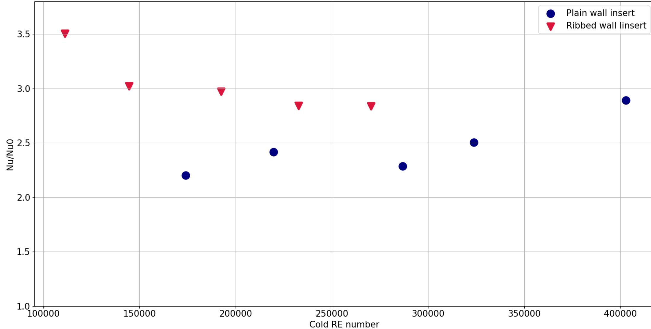
The parameter  $Nu/Nu_0$  compares the calculated test Nusselt number to a smooth wall Nusselt number calculated from the Gnielinski correlation for a fully developed internal passage with the same fluid conditions.
