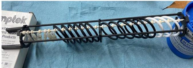
O-ring compression jig used in sCO<sub>2</sub> exposure; 25% deflection shim used
