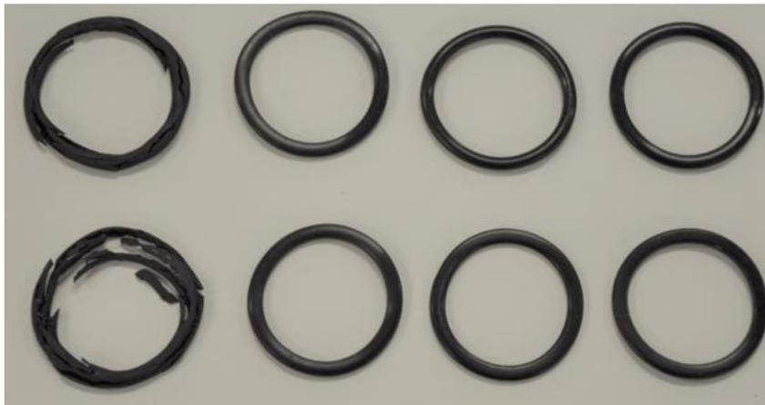
Picture of whole O-rings after compressed exposure to 20 MPa sCO<sub>2</sub> at 100°C: from left – top row: Viton sample 1, Buna N, EPDM, HNBR; bottom row – Viton sample 2, EPR, Neoprene (uncoated) and Neoprene (coated)
