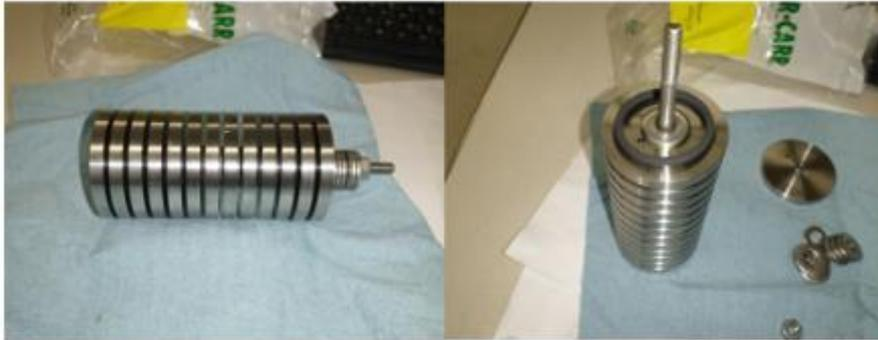
Compression fixtures designed to hold the O-rings inside the sCO<sub>2</sub> autoclave
