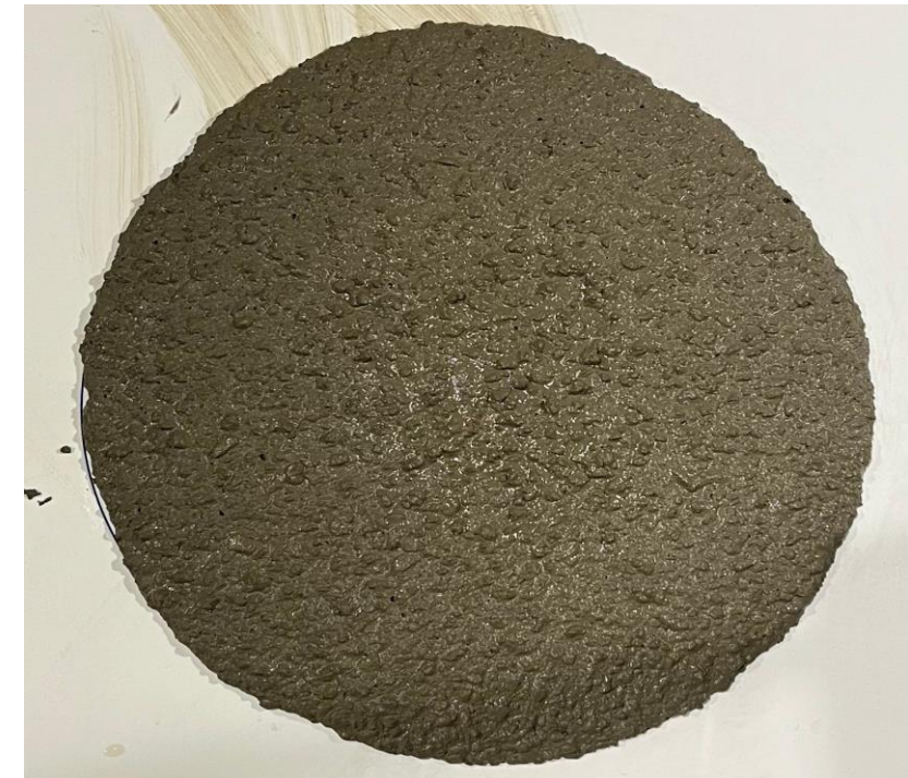
Slump flow test for an L40 mix. High stability with no segregation was observed.
