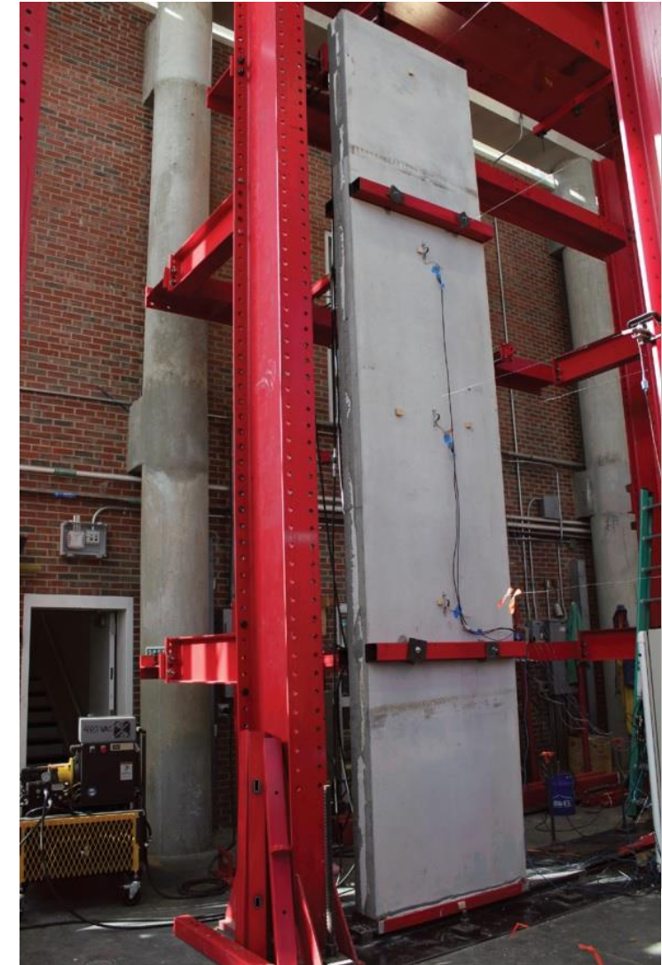
Nafadi et al. (2021). "Long-term behavior of precast, prestressed concrete sandwich panels reinforced with carbon-fiber-reinforced polymer shear grid" PCI Journal.
