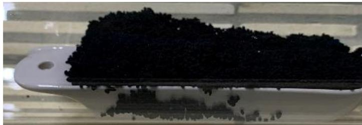
Post-test material with carbon buildup
