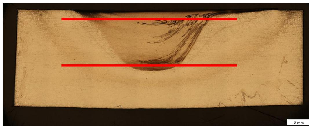
Creep Testing Coupon Material Area
