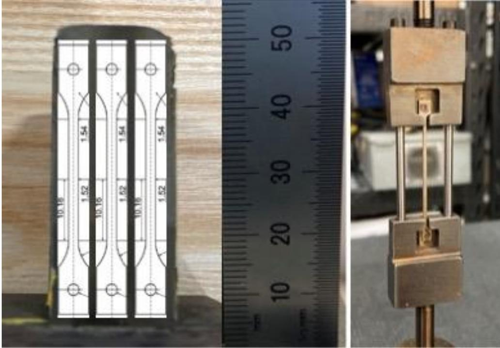
Non-standard tensile samples extracted (SS1 gage length and SSJ3 grip geometry)
