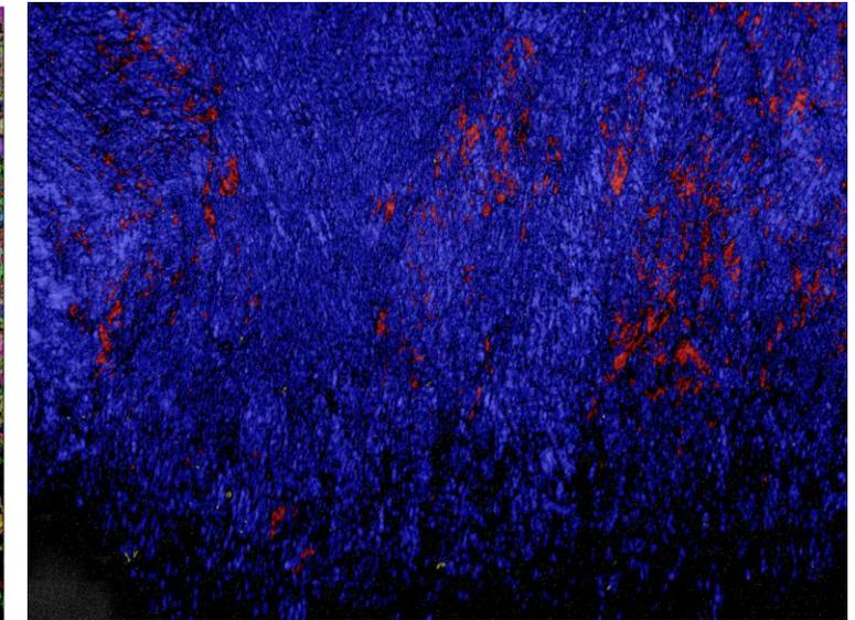
Failure occurs in the dual-phase region near the SS347H side of the joint
