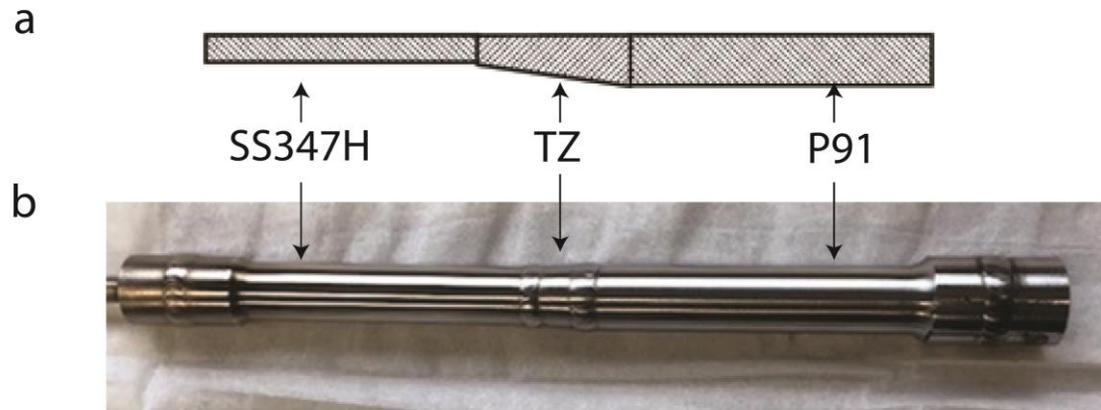
Larson-Miller approach used to determine creep stress of 165MPa for SS347H and 103MPa for G91 for a stress rupture time of 500h at 650 °C
