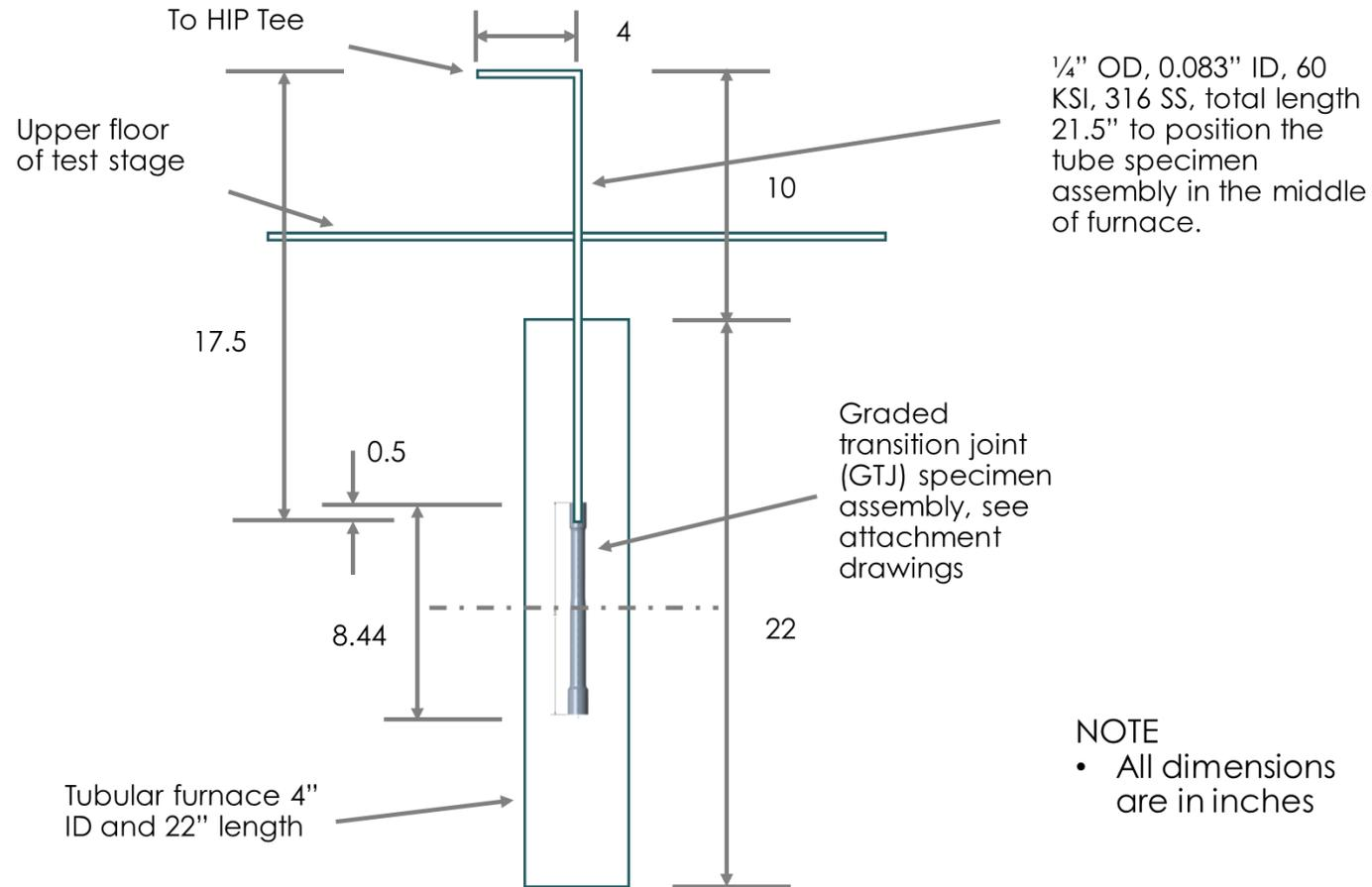
1/4" OD, 0.083" ID, 60 KSI, 316 SS, total length 21.5" to position the tube specimen assembly in the middle of furnace.
