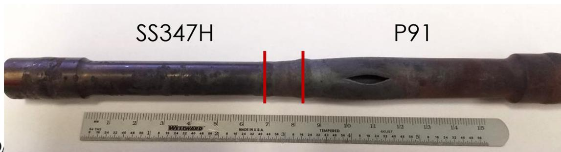
Different cross-section thicknesses used to equate rupture time in all sessions
