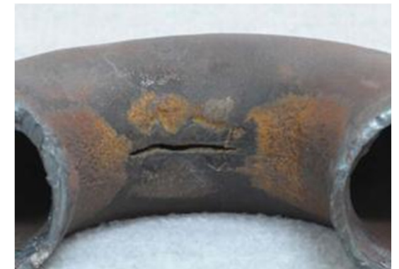
Stress corrosion cracking
