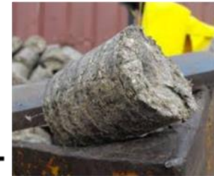
Densified biomass with less water uptake
