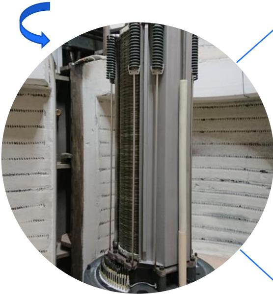
**Solid oxide stack is a common platform**
