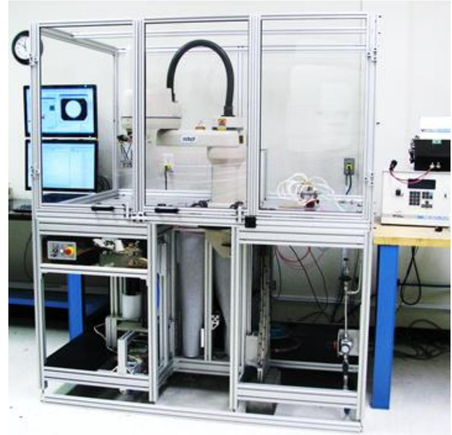
**Automated screen printing, drying, cell QC, stack firing, and stack handling equipment**
