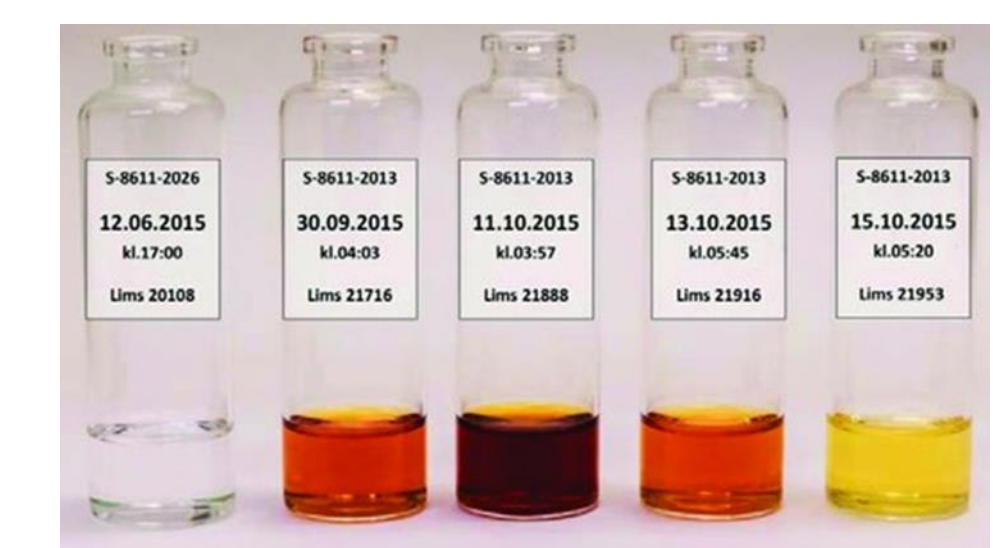
Figure 2. Examples of an amine solvent system degradation over time. 9
