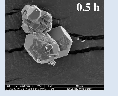
Rod-like gypsums are fully transformed into well-faceted calcite crystals within 30 min of reaction time under mild synthesis conditions
