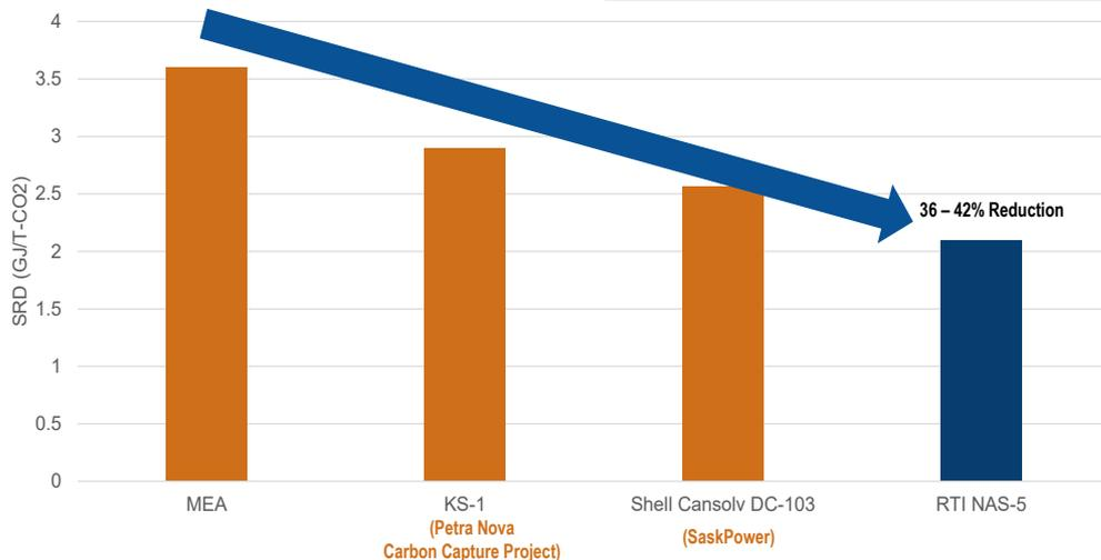
RTI evaluates wide range of low-cost, commercially-produced amines with the following characteristics:
