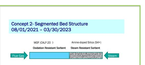
Segmented bed concept matches the best sorbent to the position of the bed (based on RH and Temperature profile)
