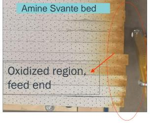
Only a small portion of the bed is showing significant degradation
