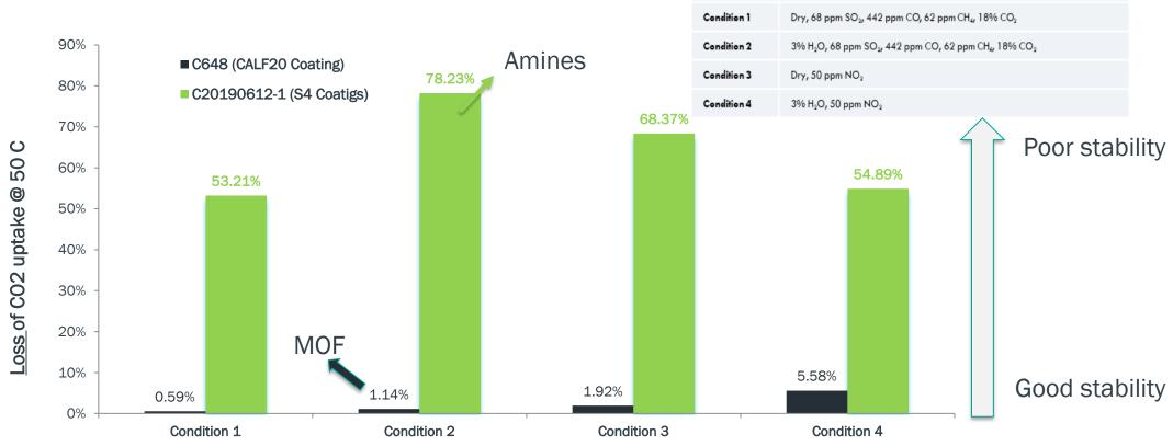
MOF (Calf20) laminate shows excellent tolerance to SOx and Nox, which opens this utilization for harsh flue-gas environments (ex., Cement)
