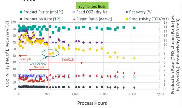
Some drop in capacity was observed because of the effect of contaminants on the amines-based sorbent.
