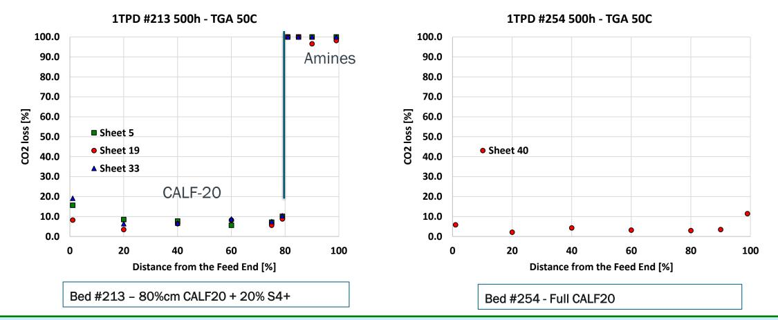
This bed is showing high CO2 capacity loss of the amines based section because of the presence of contaminants higher contaminants. MOF material is showing negligible lost after 500 hrs operation.
