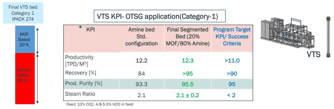
These VTS results allow confirming that the model and test results were aligned. The PDU bed geometry was finalized at this stage, and the PDU testing is to study the bed lifetime of the Segmented bed on the OTSG application.
