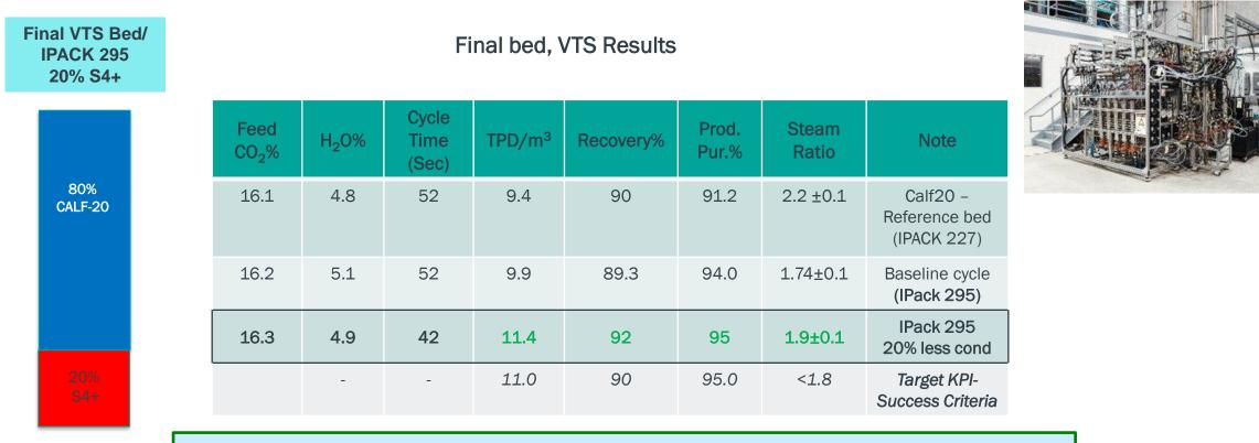
IPACK 295- segmented bed showing better performance as reference CALF20 with 20% less conditioning (lowering OPEX and CAPEX)
