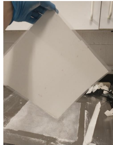
12" x 12" laminate after drying
