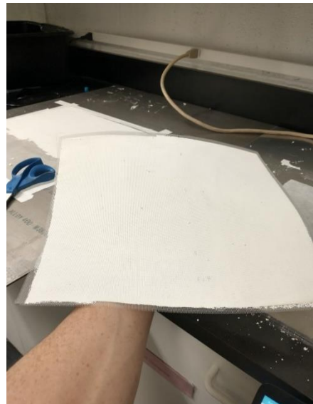
12" x 12" laminate after drying
