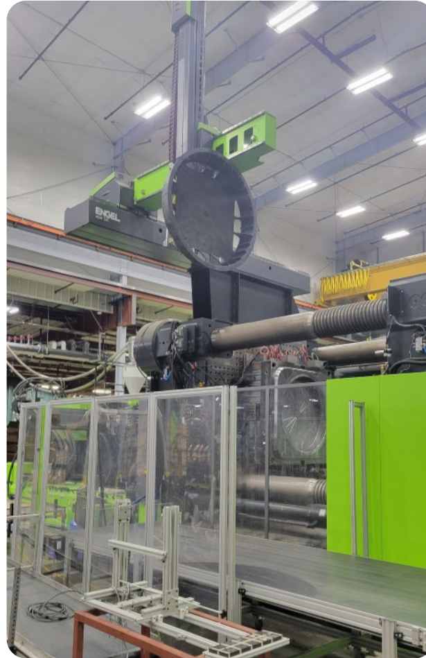
Injected molder – production run of commercial plastic housings
