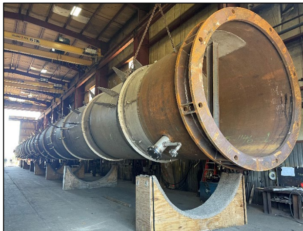
Absorber column at fabricator shop
