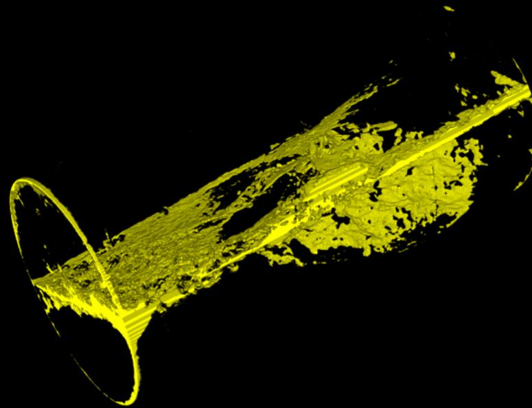
Marcellus Fracture and Reacted Matrix at Experiment End
