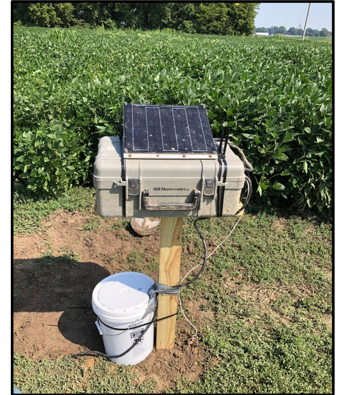
NETL seismometer at Prairie State CarbonSAFE Site, Washington County, IL
