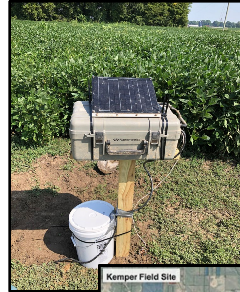
NETL seismometer at Prairie State CarbonSAFE Site, Washington County, IL
