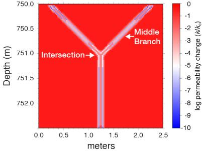
Simulation results showing patterns of permeability change caused by  $CO_2$  mineralization in a basalt fracture for a moderate permeability-porosity coupling
