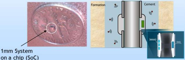
(Left) Sensor systems that communicate wirelessly with casing collars, (Right) providing real-time distributed sensor measurements in the casing annular space, and the formation
