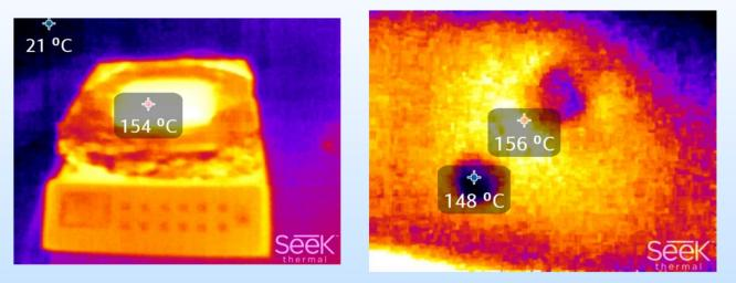
Higher temperatures did not permanently damage the chip, it would begin communicating again afterwards.
