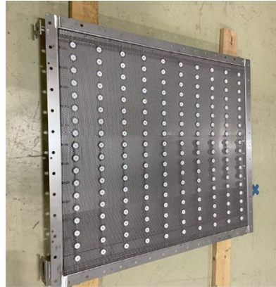
Cathode current collector and GED support plate with the CO 2 support plate underneath (1.5 m 2 )
