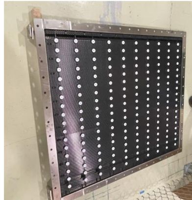
Anode (plate coated with MMO) plate with the anolyte flow assembly underneath (1.5 m 2 )
