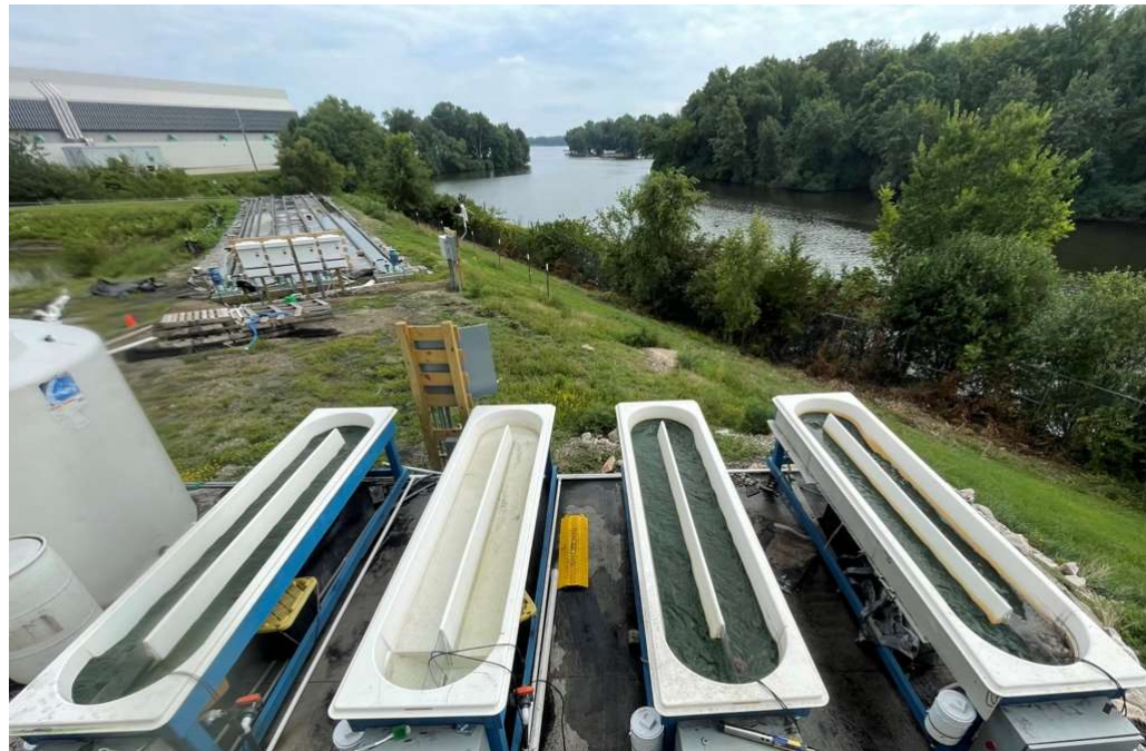
Small Raceways Used for Culture Upscaling
