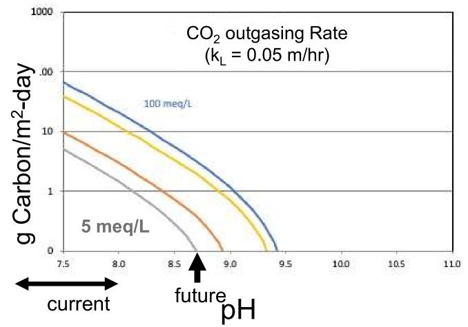
Increasing pH and increasing alkalinity greatly reduces CO<sub>2</sub> outgassing.
