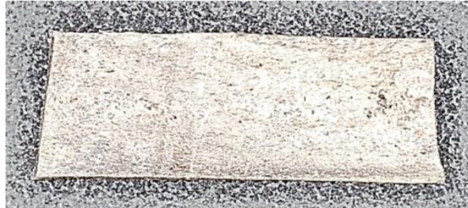
Optical photos of flexural specimens, manufactured using one-stage molding parameters
