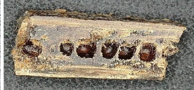
Optical photos of flexural specimens, manufactured using one-stage molding parameters
