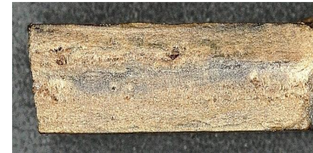
Cross-section of LPC's manufactured using two-stage molding parameters
