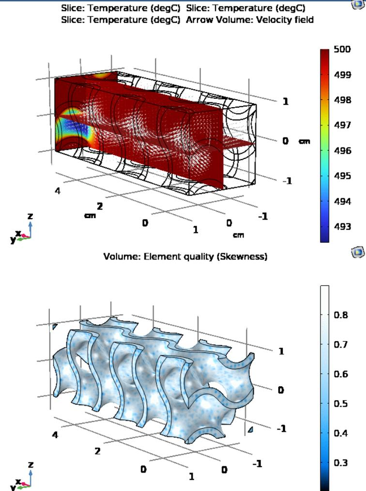
Fig. 8 – (b) Preliminary temperature profile results on a 3x1x1 HX model.
