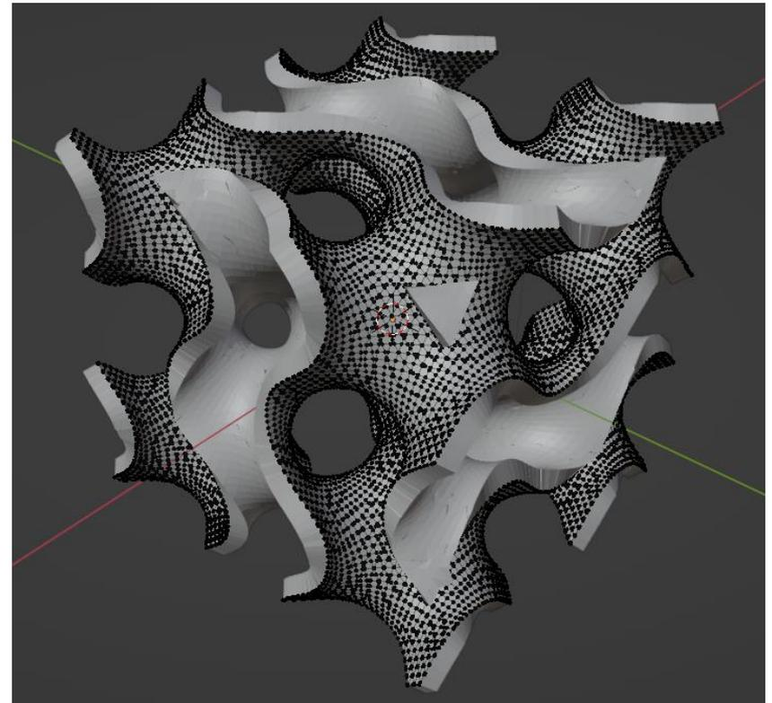
Fig. 2 – A TPMS example named gyroid, generated using MathMod and modeled in Blender
