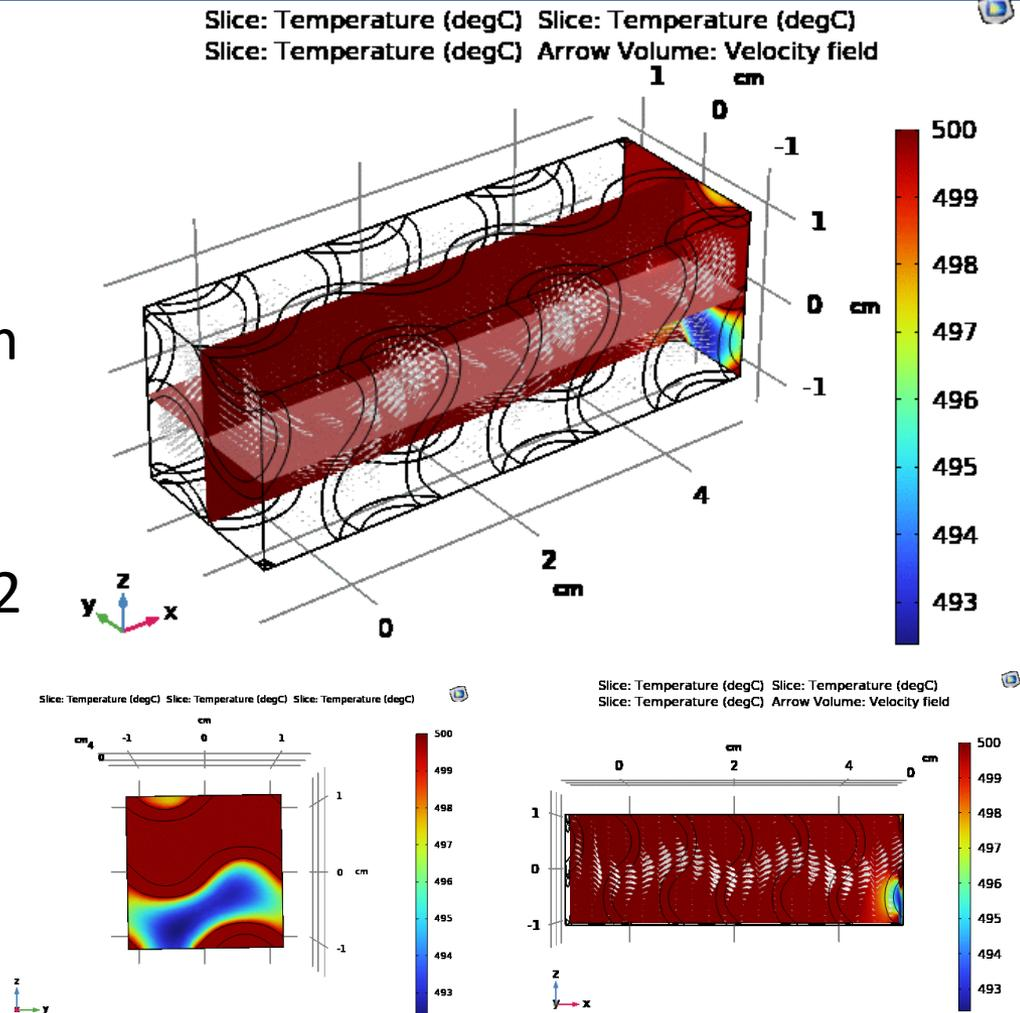
Fig. 8 – (a) Preliminary temperature profile results on a 3x1x1 HX model.
