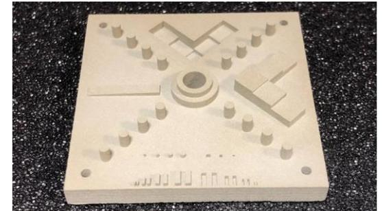
Fig. 4 – Ceramic AM samples. Images by [Kelly J. et al.]
