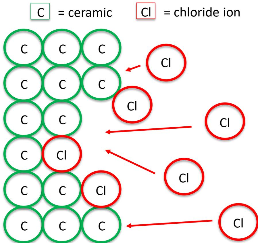
Fig. 5 – Simplified representation of corrosion on a non-oxide ceramic due to a  $\text{KCl-MgCl}_2$  salt. Image adapted from [Bell et al. '19]
