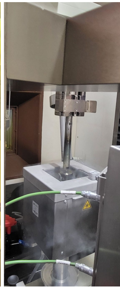
Cryogenic temperature ( \sim 80\text{K} ) was performed at 5 \times 10^{-4}/\text{s} displacement rate on 316SS specimens (S1).
