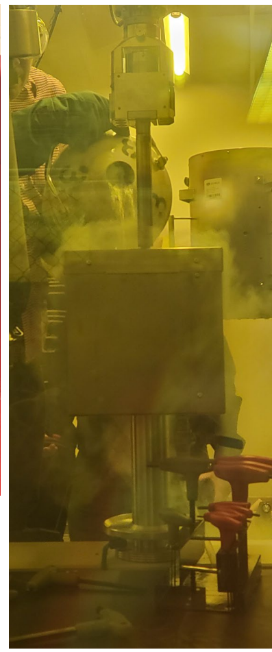
(left) J. Justice is having fun with manipulators installing specimen on Zwick Roell AllroundLine 2020 THW while \text{LN}_2 bath is being filled by the O. Anderoglu (right)
