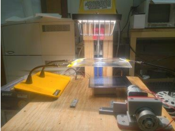
Figure 11. Fresnel Lens at 3 inches with respect solar cell
