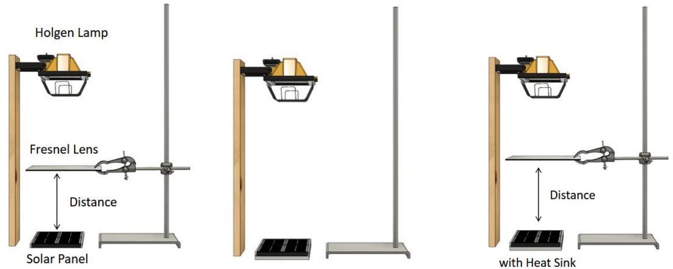
Figure 2. How we tested the viability of a Fresnel lens
