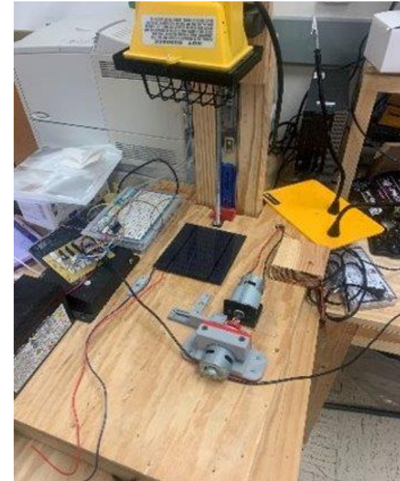
Figure 4. Solar panel in normal conditions, 13.5 inches from the lamp
