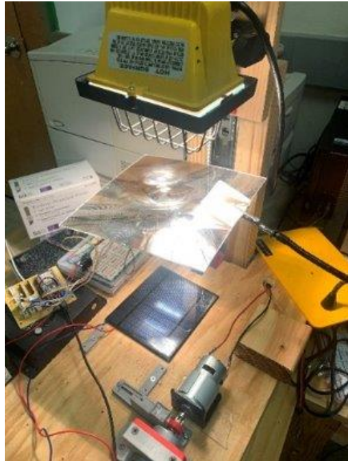
Figure 5. Here we have the Lens 9 inches away from the PV
