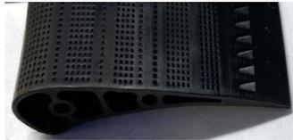
Complex geometries including transpiration and film cooled configurations are possible with the AM PDC processes developed
