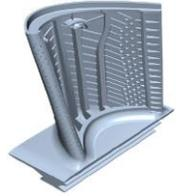
**Motivation: enable superalloy-like cooling features in CMC-like materials to enable higher temperature operation**
