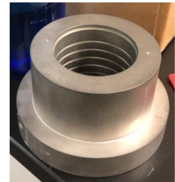
**Valve components, drum blades and NDE standards printed on new Binderjet process to establish the cost/resolution evaluation. Preliminary trials done with 316 and IN718 (>99% density)**
