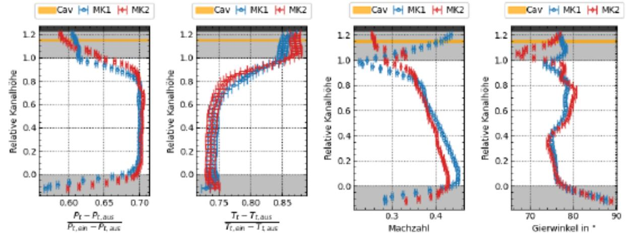
The pressure losses are shifted to the outer side wall which clearly indicates the impact of the bypass blades.
