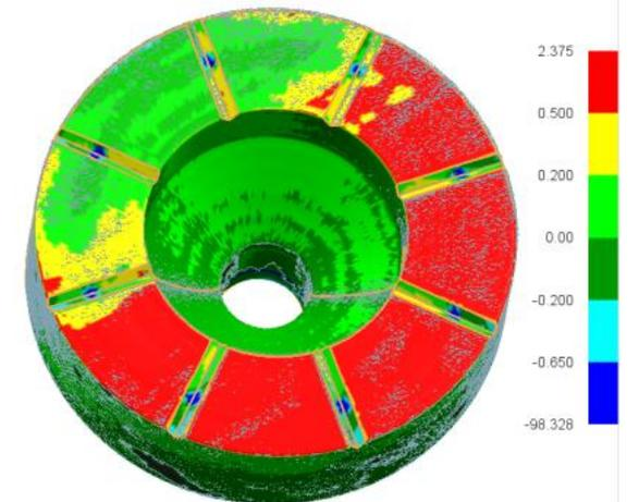
Bionic valve deviation is likely due to inaccuracy of measuring main axis direction
