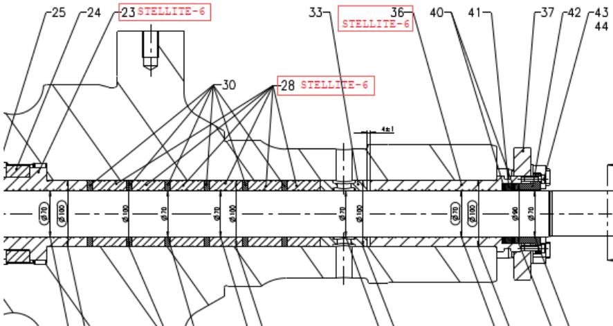
HP Stop Valve cross-section
