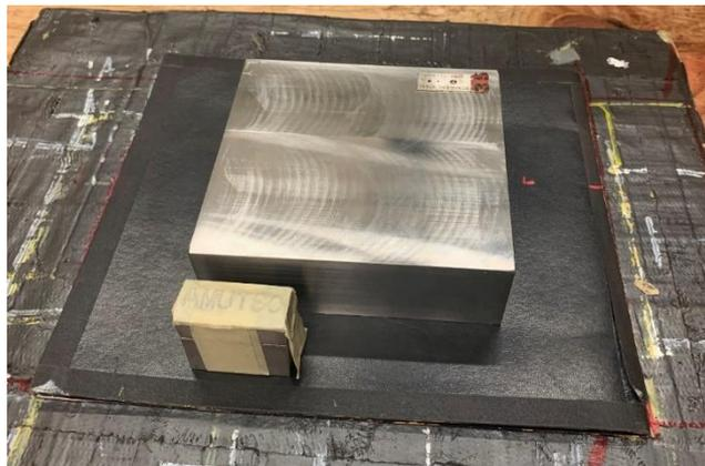
AMUTSO block, ASTM IQI plaque and film arrangement
