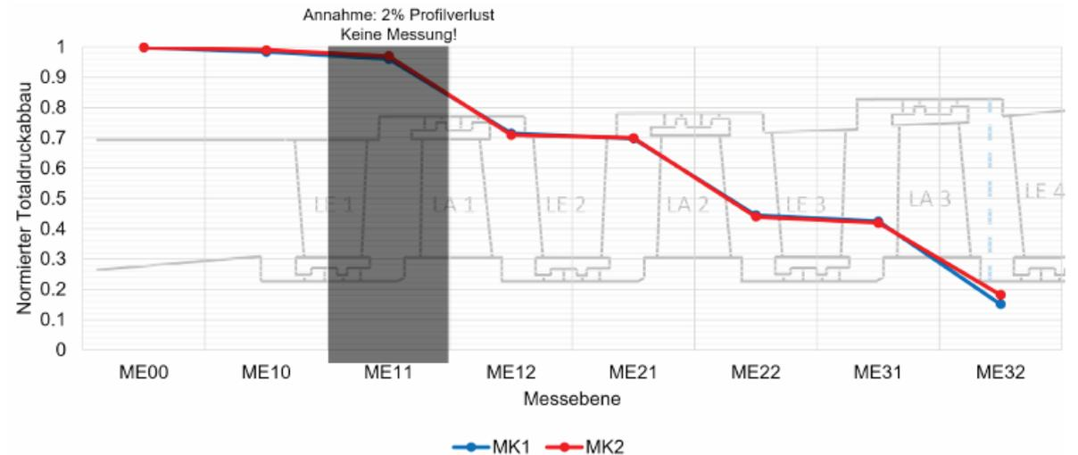
A lower normalized total pressure loss or profile loss of 0.7% is observed with 1<sup>st</sup> iteration
