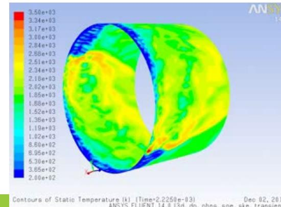
Temperature contours from simulation of RDE operating on H2-Air (NETL).
