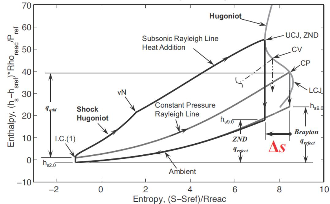
H-S diagram comparing constant pressure combustion (Brayton) cycle to near-constant volume combustion (Humphrey) cycle.
