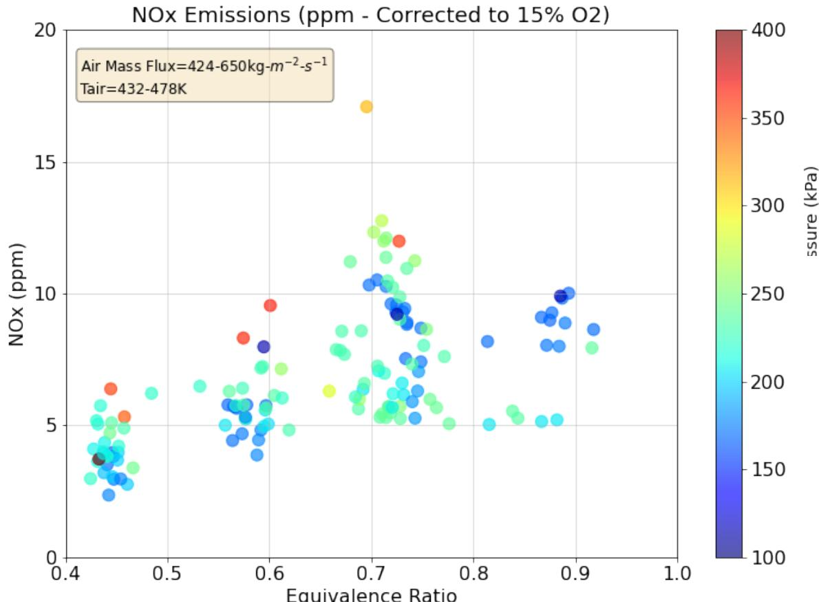
$$\text{Oxygen referenced conc.} = \text{Measured conc.} \times \frac{20.9 - \text{Oxygen Reference value} (\%)}{20.9 - \text{measured oxygen} (\%)}$$
