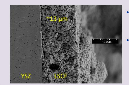
Cathode thicknesses less than 20 µm can be achieved • Potential to manufacture varied microstructure in z-
