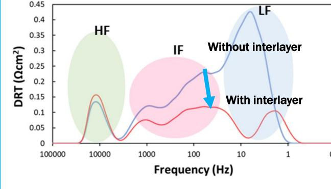
The optimized interlayer reduces both ohmic and polarization resistances by enhancing interfacial condition, facilitating gas diffusion and charge transfer reaction at low operating temperatures (i.e., ≤ 600 °C)
