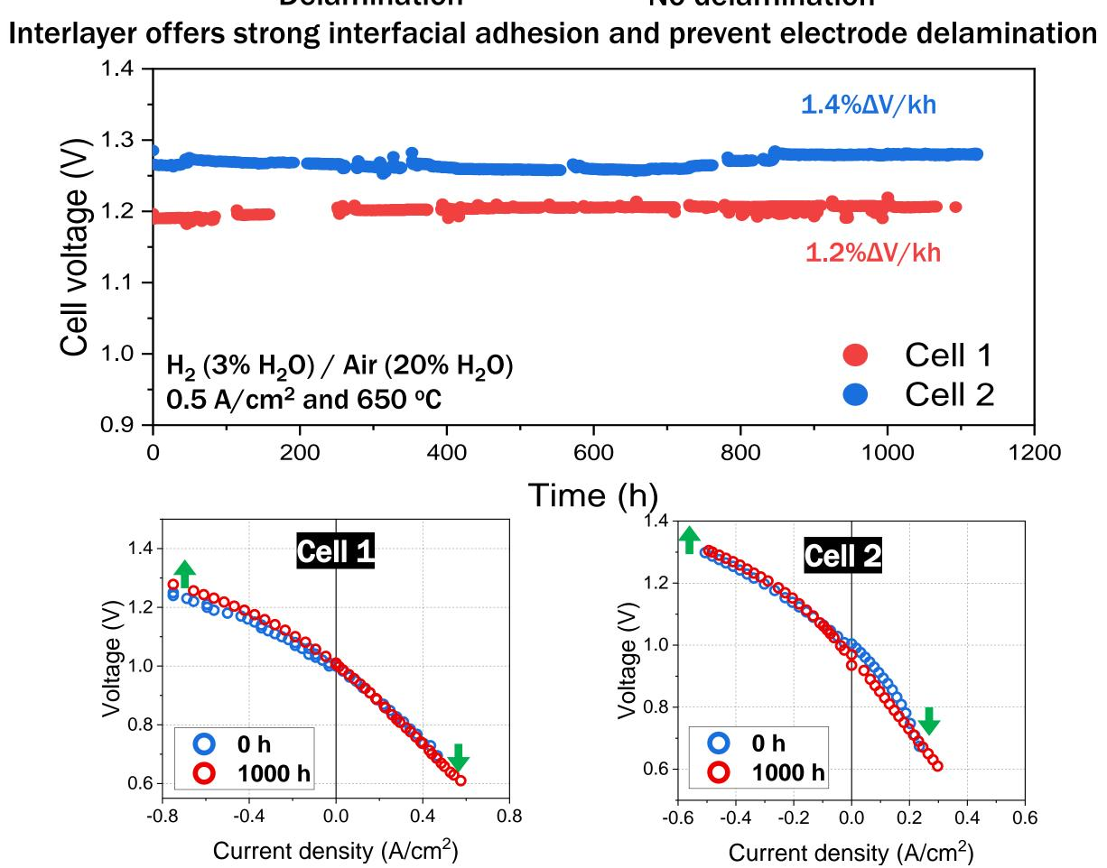
The 1100-h operation demonstrated excellent long-term stability of large cells with an interlayer
