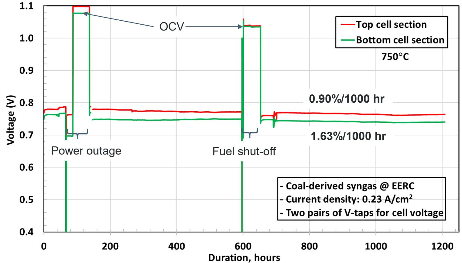
Long-Term Durability Test under Constant Current at 750°C.
