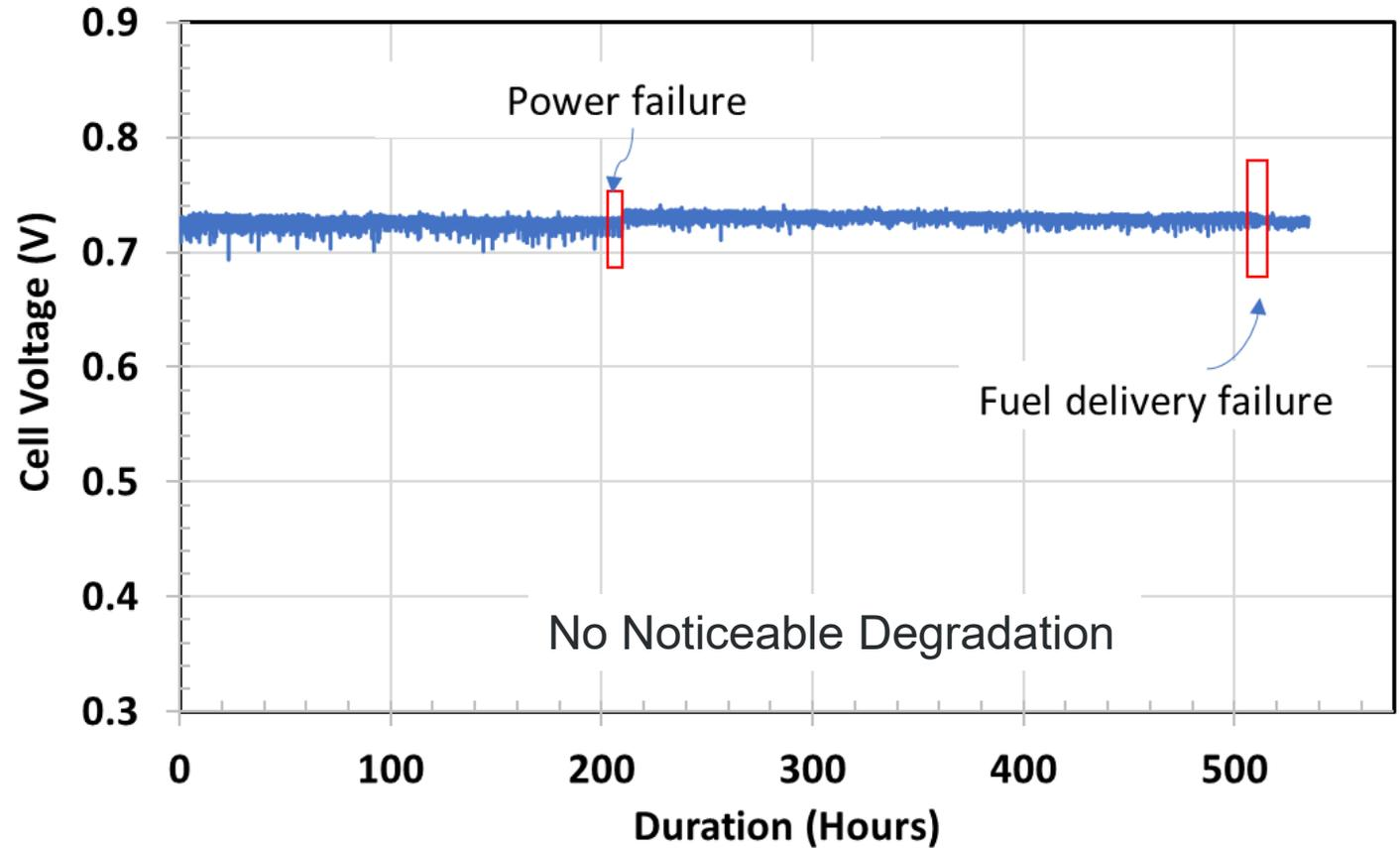
Long-Term Durability Test Using Natural Gas Fuel
