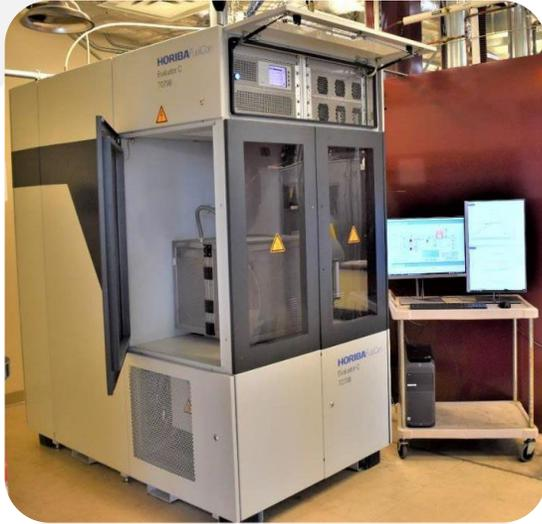
1-kW Stack Test Station
