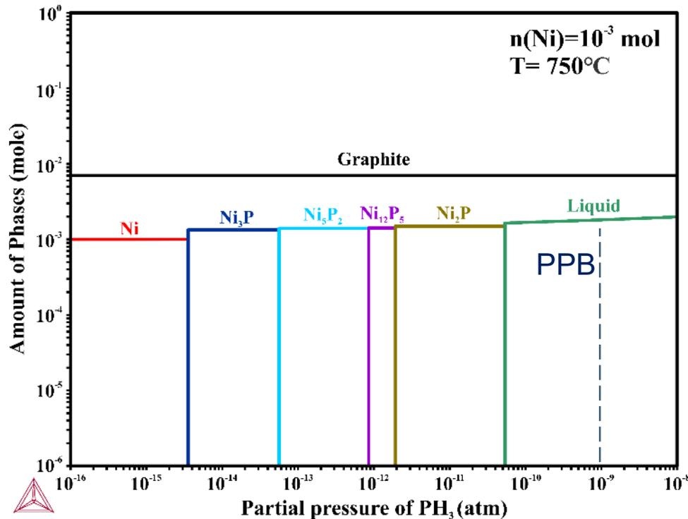
Nickel Phosphide Formation vs. Phosphine Partial Pressure
