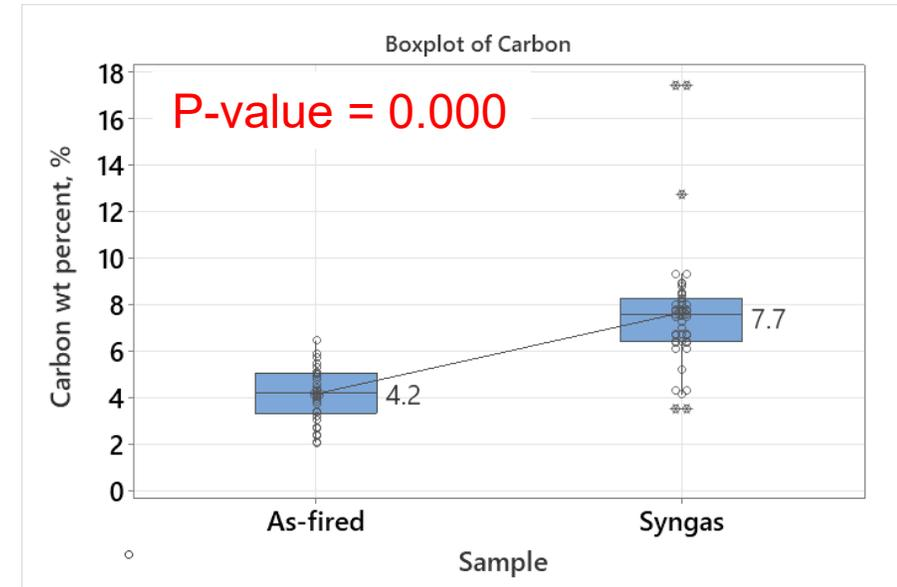
Statistical Data Analysis of Carbon on Anode Surface
