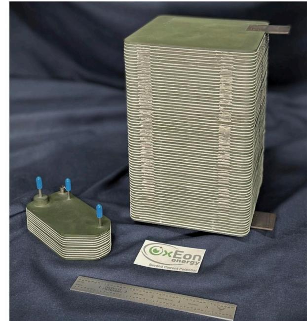
MOXIE scale stack (left) and demonstration system scale stack (right)
