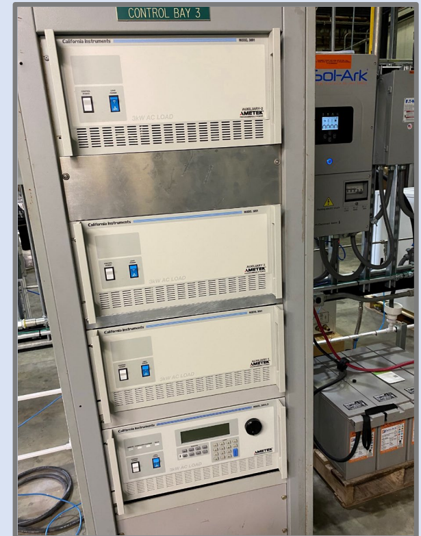
California Instruments 3091LD AC Electronic Load in foreground and Sol-Ark hybrid inverter as “AC Coupling” in background
