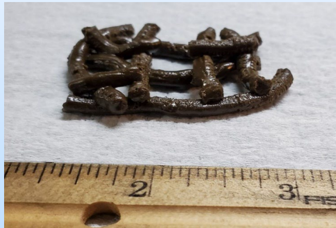
3 Layers of Stacked Filaments after 250°C Cure
