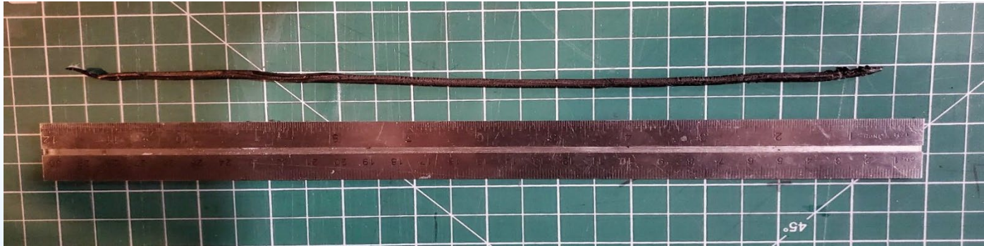
3 mm Filament of B215 Resin and 67% Fly Ash
