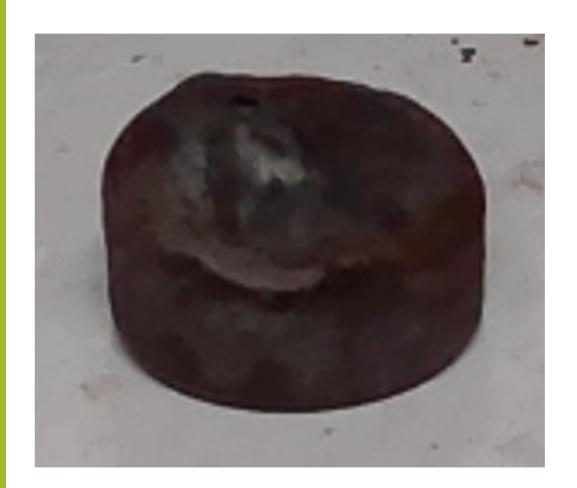
Heated sintered sample to 1300C. Sample melted and became glassy and very hard. Couldn't grind it flat for compression test
