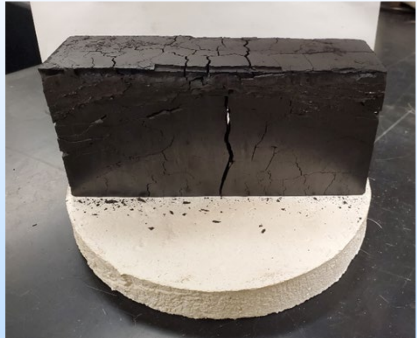
Preliminary pre-sintered LIG2 brick (left), and post-sintered LIG2 brick (right). Second attempt of LIG2 brick fabrication.
