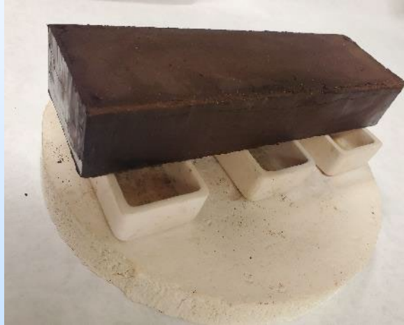
Preliminary pre-sintered LIG2 brick (left), post-drying (middle), and post-sintered LIG2 brick (right). 9 th attempt of LIG2 brick fabrication.
