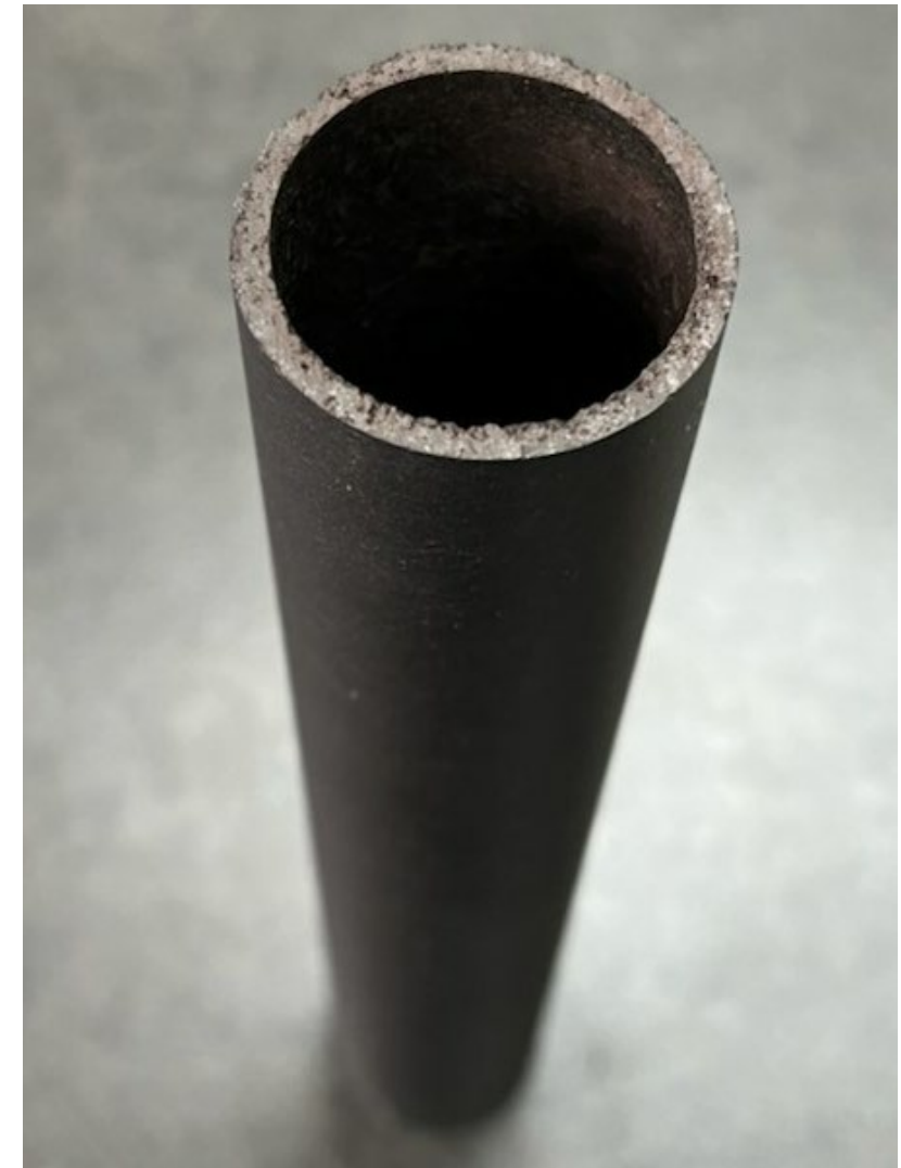
1¼ in Schedule 40 PVC pipe made with CPC formulation
