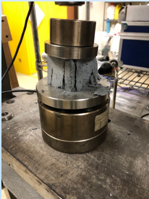
X-MORTAR Compression Cubes
