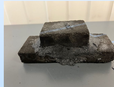
Ceramic X-BRICK Components Bonded with X-MORTAR
