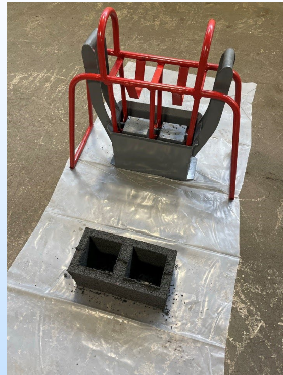
CART Improved Process for X-MATRIX Blocks compared with utilizing a wooden mold
