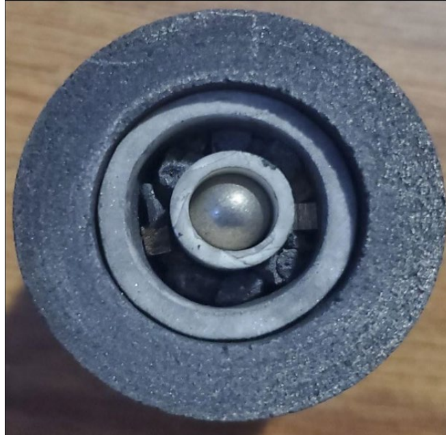
Reactor crucible packed with bulk carbon prior to operation
