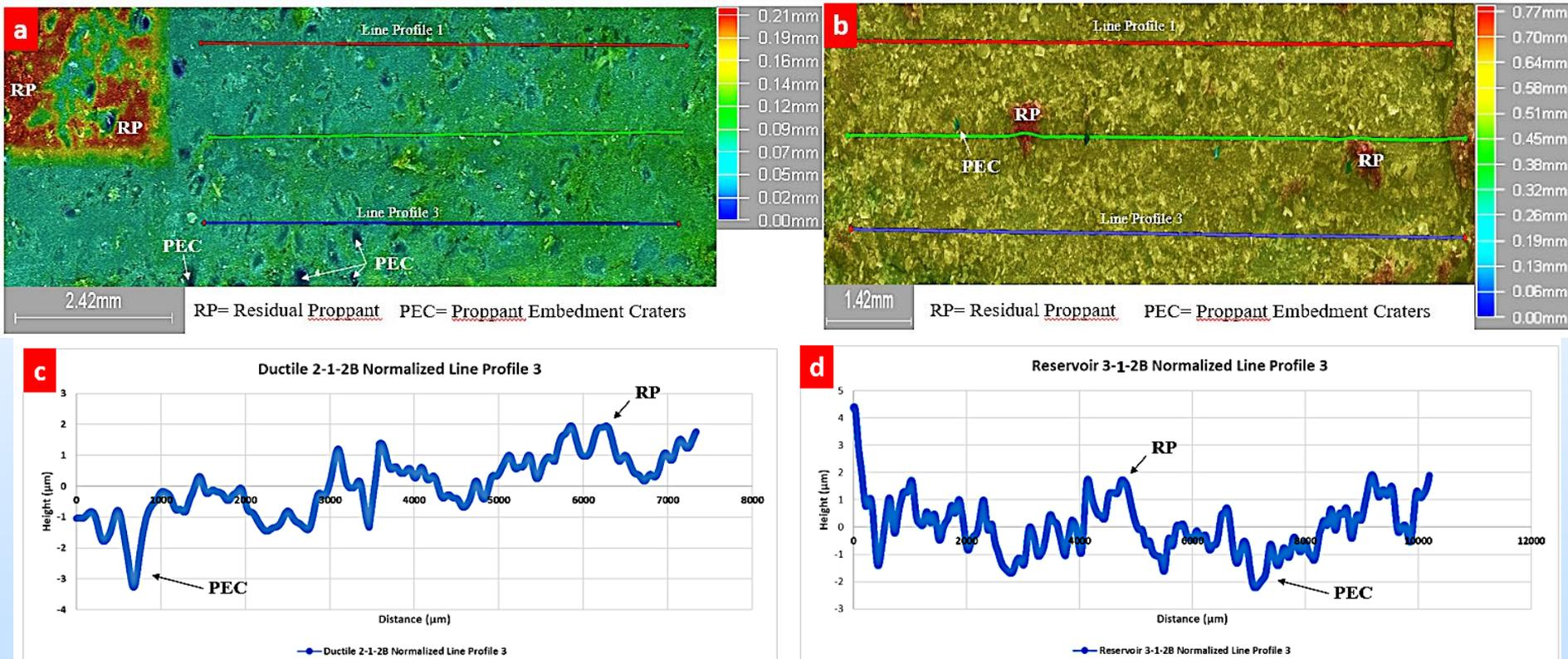
Optical microscopy showing effect of proppant embedment on fracture wall surface roughness (a,b)
