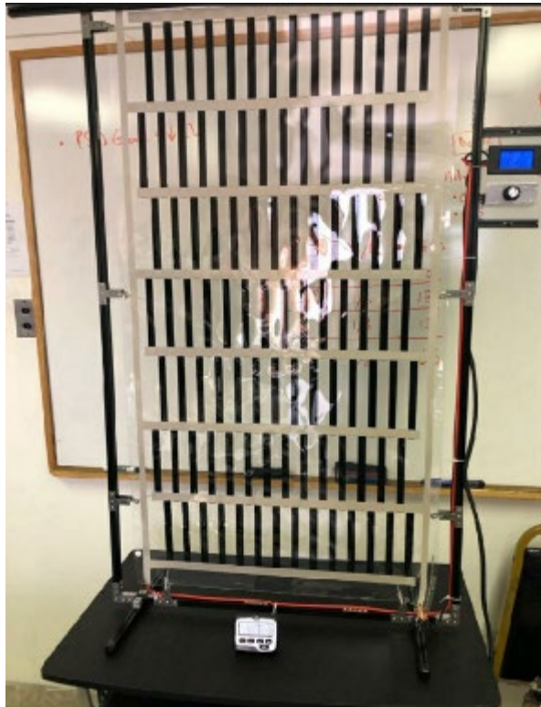
Prototype of 2' x 4' Commercial-Scale Wall Heating Panel
