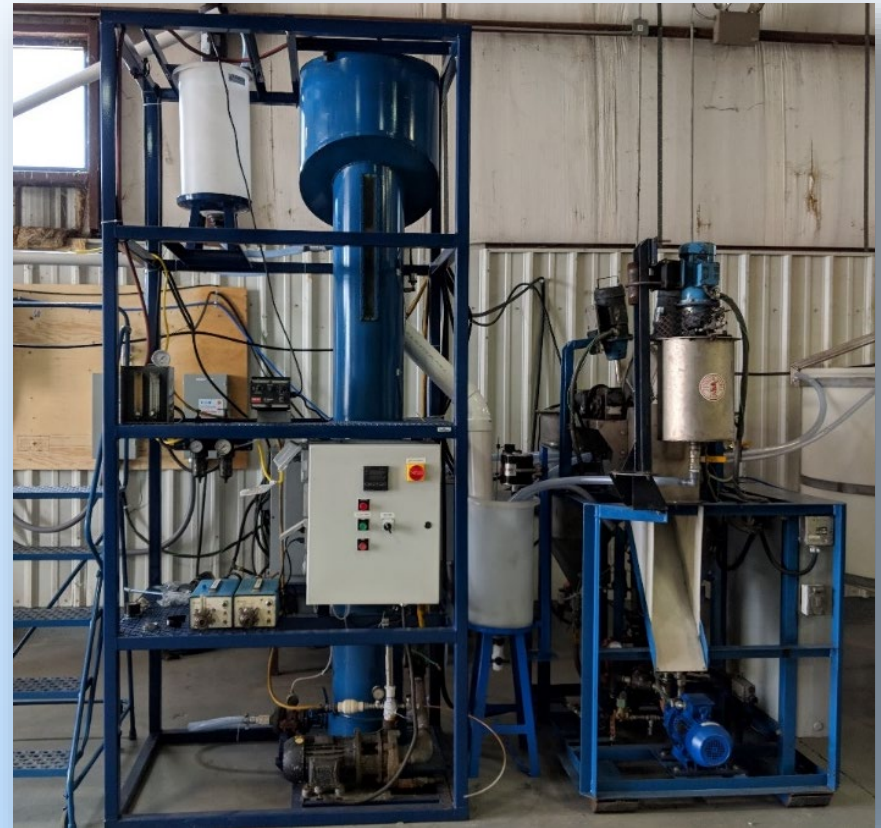
Column Flotation Circuit
