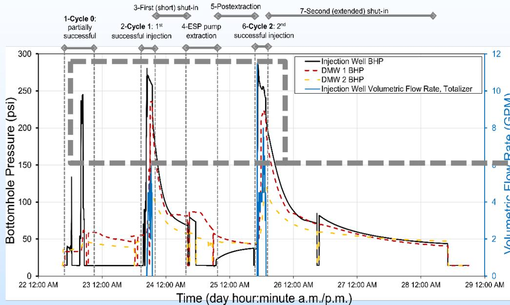
Large change of fracture permeability during fracture reopening (Step 2)
