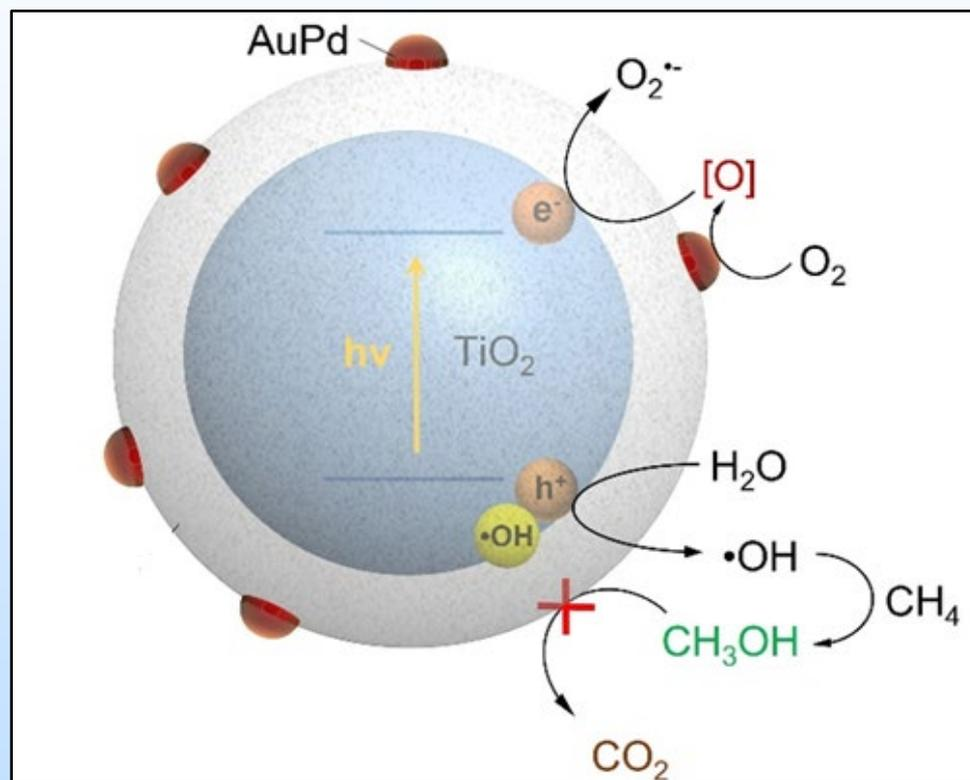
$\text{TiO}_2$ -based designed photocatalyst
