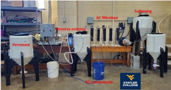
Laboratory at WVU I Dr. Lance Lin Builds off previous FECM/NETL grant: Co-treating Cooling Tower Blowdown and Produced Water, Dr. Harry Finklea, Co-Pl
