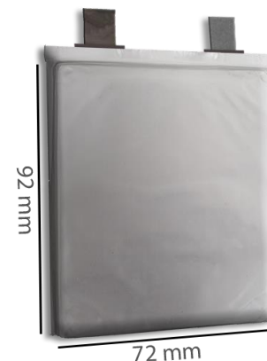
PSI's 13,000 mAh Commercial Pouch Cell
